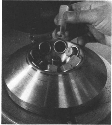
Figure 30. Placing the assembly in the 12,000 r.p.m. micro centrifuge
